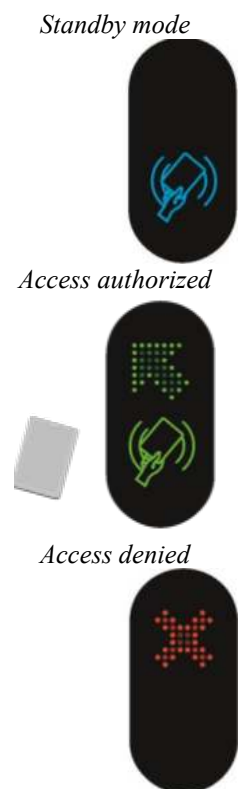
Fig.8 - LED display status lights
